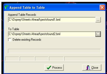
Ideally the target layer should have the same structure as the original layer. However it is possible to append to a layer of a different structure provided some fields have the same name and are of the same type as the original layer.
